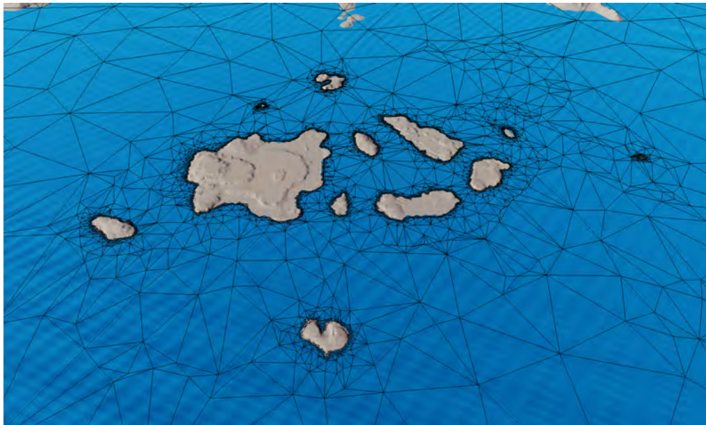
Figure 3: A visual representation of the coarse mesh (black triangles) for an example scene (white terrain) generated using the method described in section 4.2.2. Note how the sampling approach maintains a high density of vertices along the shoreline while not over-sampling the region of flat bottomed shallow water in between the islands.
